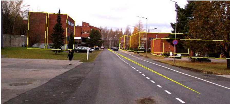
Figure 3-3. The camera location is shifted one meter. Error is clearly visible and easy to correct interactively. The image is taken with a normal digital camera that has been calibrated.
