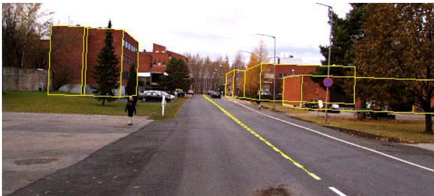
Figure 3-4. Exterior orientation of the image is solved by interactive method. Simplified 3D vector data projected onto the image fits quite well.
