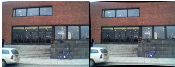
Figure 3-2. Left image: original image taken with a mobile phone camera. Right image: the same image after lens distortion removal.
