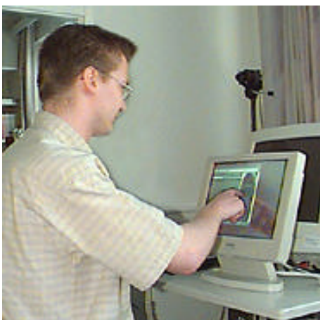
Figure 2. Touch screen being used with a PC emulation of a mobile phone.
